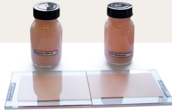
Figure 1: Films of pigmented binders; left: base formulation 1 with continuously produced product; right: base formulation 2 with suspension polymer
